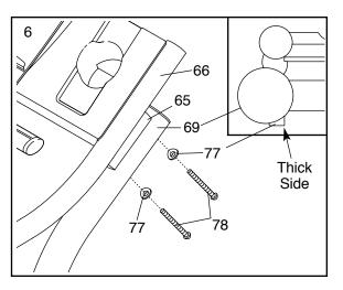
7. Make sure that all parts are properly tightened before you use the treadmill. Note: If there is a thin sheet of clear plastic on the hood decal, remove it. Keep the included allen wrench in a secure place. The allen wrench is used to adjust the walking belt (see page 24). To protect the floor or carpet from damage, place a mat under the treadmill.
